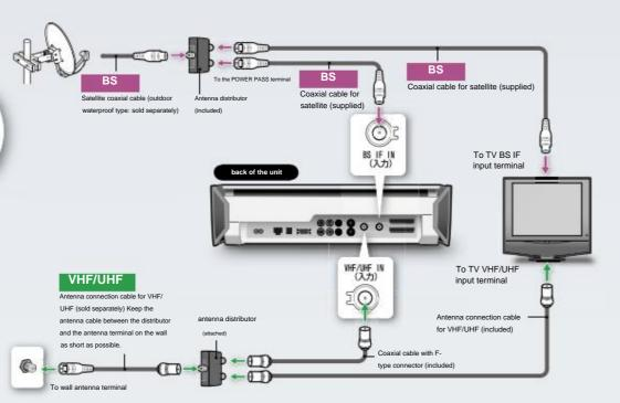
When supplying power from this unit to the BS antenna, connect the terminal labeled POWER
